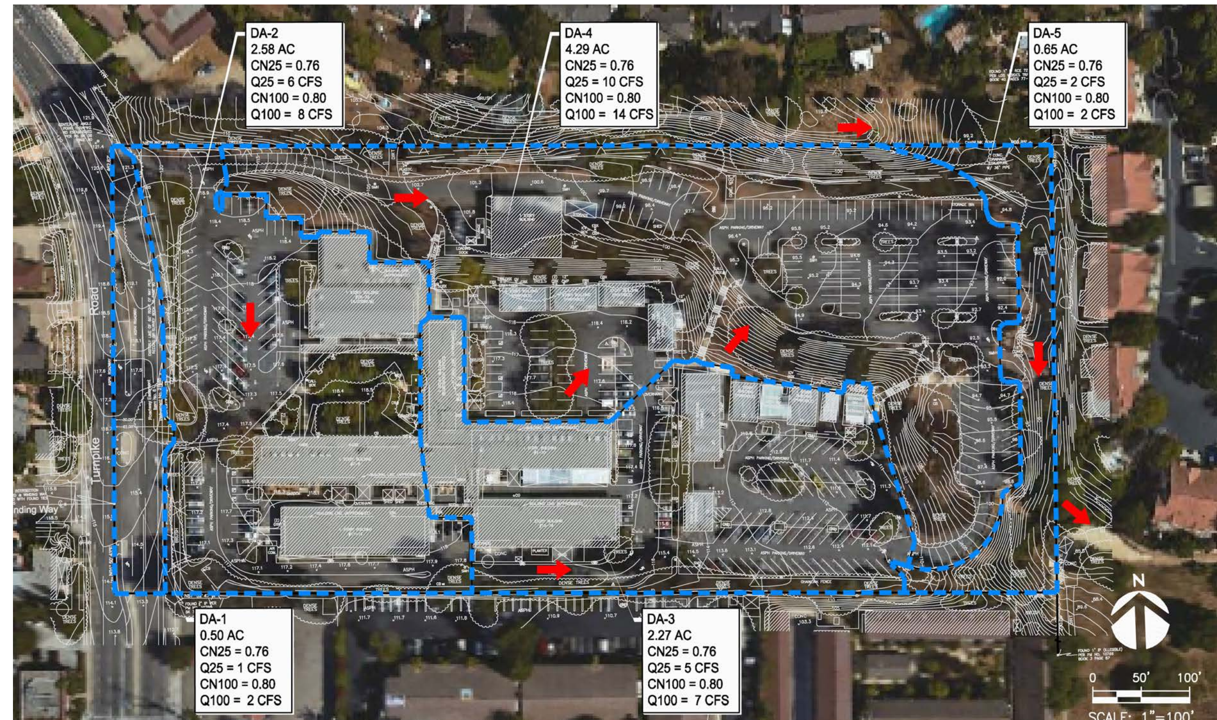
Figure 3.2.3 Existing Drainage Areas
